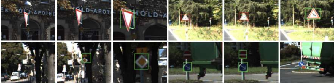
Fig. 1. Examples of traffic sign detections from a single-image based detector. Red boxes denote incorrect classes and green boxes denote correct classes, note that many missed detections and incorrect detections with wrong sizes and locations exist.
